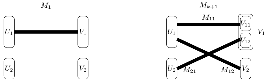
Fig. 1. G is the input graph. On the left we show the matching constructed in the first pass. On the right we show the matching constructed in the k + 1 st pass.
